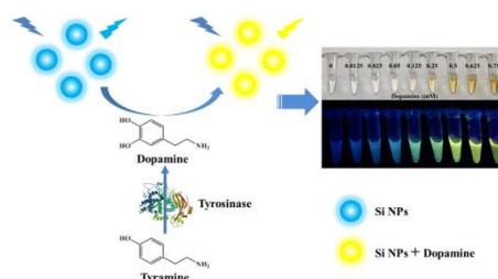
Fig. 1 Schematic illustration of the Si NPs for tyrosinase activity detection
