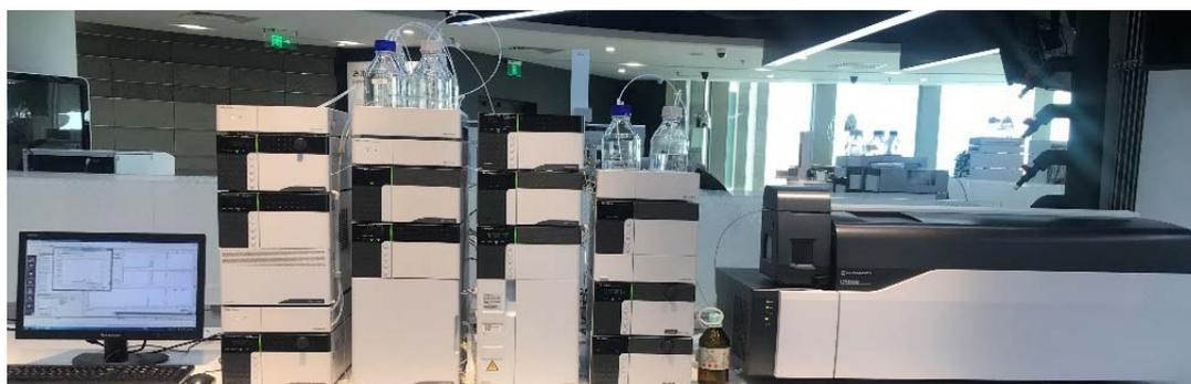
Fig. 1 Diagram of SFC-LCMS system
