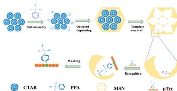
Schematic representation of the synthesis and enrichment process for the molecular imprinted mesoporous silica nanoparticles
