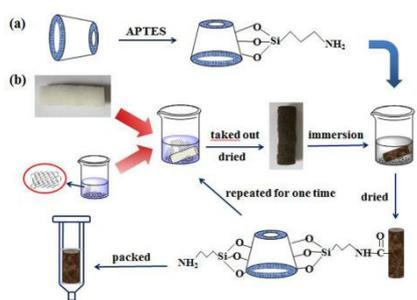
Fig. 1 Schematic illustration of the preparation process of 3D  $\beta$ -CD/GO-wrapped MF.
