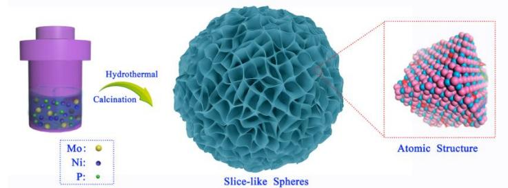
Figure 1 the synthetic process and structural characteristics of Mo-Ni<sub>5</sub>P<sub>4</sub>
